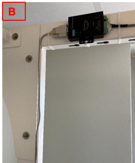
3. Attach the Serial Converter to the stand using one (1) of the included Cable Ties (C).
