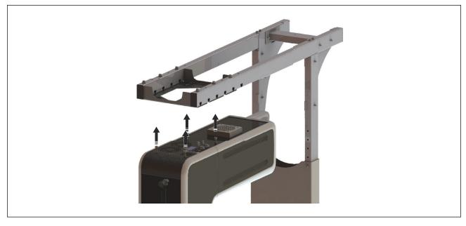
8. Insert the 4 bolts into the 4 holes and push the ITCU into position. Refer to the *Installation manual - Single Head Stand* for information on how to make the ITCU level and how to put the embroidery machine in position.
