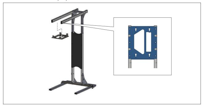
3. Install the bolts, washers and nuts. Tighten the bolts with 46 Nm.
