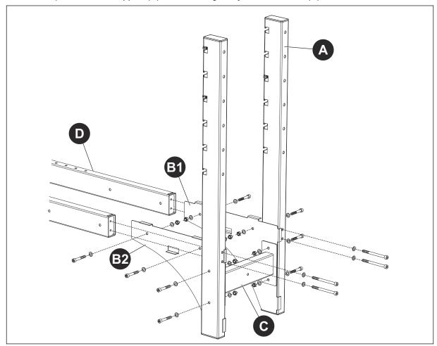
2. Install the top support plates and the mid support to the long beams. Install the height adjustment beams to the top support plates and long beams. Use the bolts, washers and nuts that was removed in step 1. The installation of the long beams is done with the same procedure as the standard upper beams. Refer to the *Installation manual - Single Head Stand* for a more detailed instruction.
