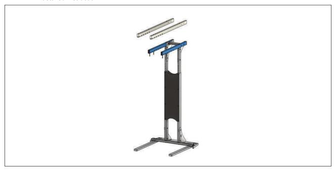
3. Put the floor stand in position, adjust the floor beams (A) if it is necessary.
