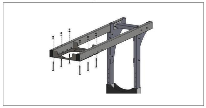
4. If the ITCU is installed for the first time, use the bolts, washers and nuts that is included with the installation kit for the single head stand and the ITCU. Install the bolts (U), the washers (Y) and the nuts (W) to the frame plate of the ITCU. Refer to the *Installation manual - Single Head Stand*.
