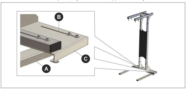
4. Put the fastener (not included) through the guide (B) as close to the edge of the base plate (C) as possible. Attach the floor stand on both sides of the height adjustment beams.
