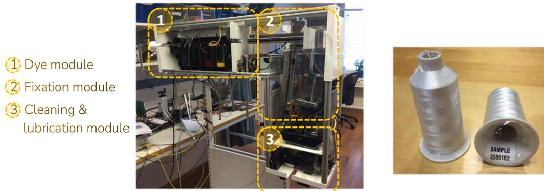
Figure 5, show parts of the Coloreel unit and the special Coloreel thread.
