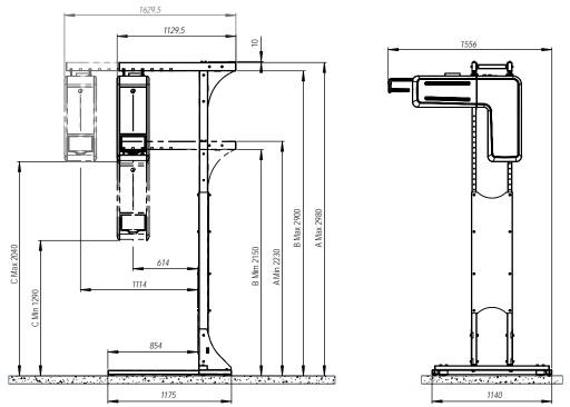
Note that the use of Long beams requires the stand to be secured to the floor. Dimension of bolt: M8. Use a large washer. Type of bolt will depend on the floor material!
